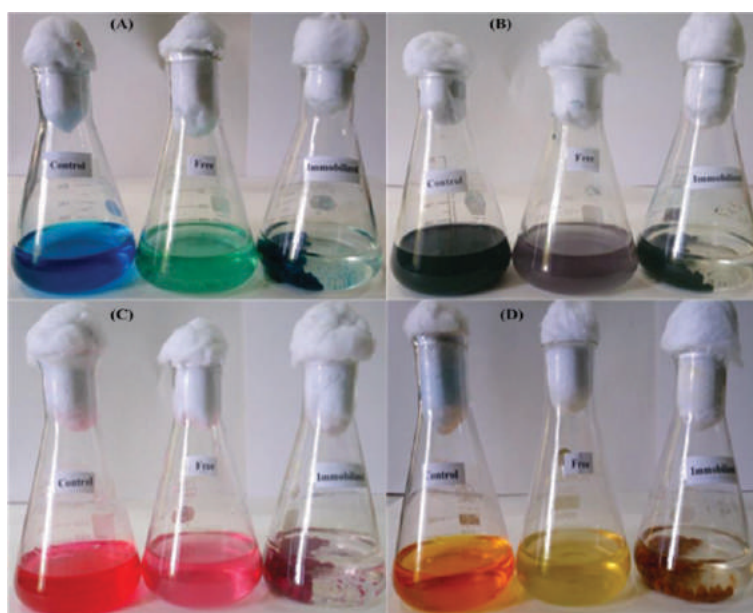
Fig.6 Visual comparison of Sandal-fix Turq blue GWF (A), Sandal-fix Black CKF (B), Sandal-fix Red C4BLN (C) and Sandal-fix Golden yellow CRL (D) dyes decolorization with free and chitosan beads immobilized MnP
